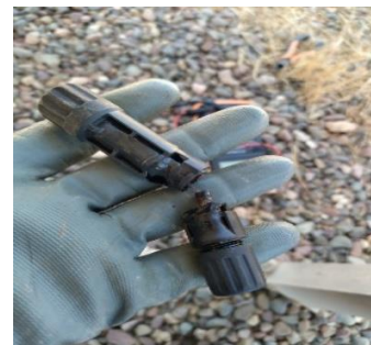
Figure 18 : Uncleaned string disconnected due to MC4 DC cable burnt
